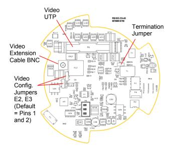
2. Set the termination jumper E1 according to the dome's position in the communications line.
